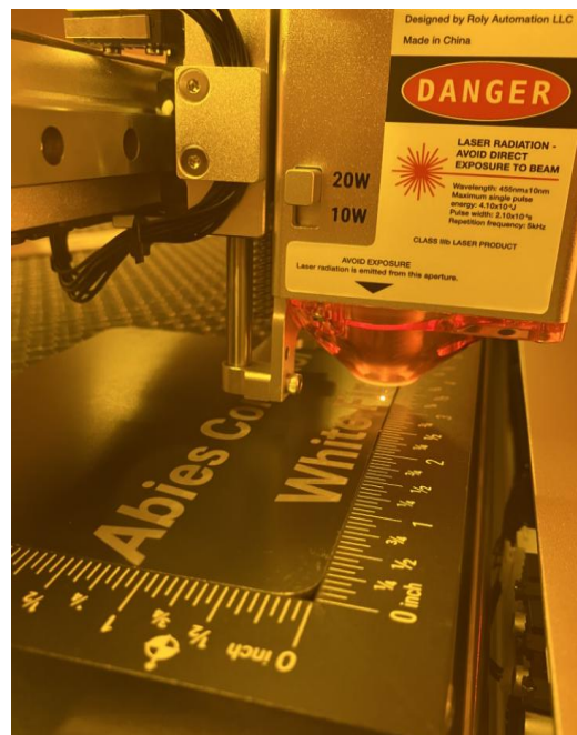
(Engraving machine making botanical markers)
