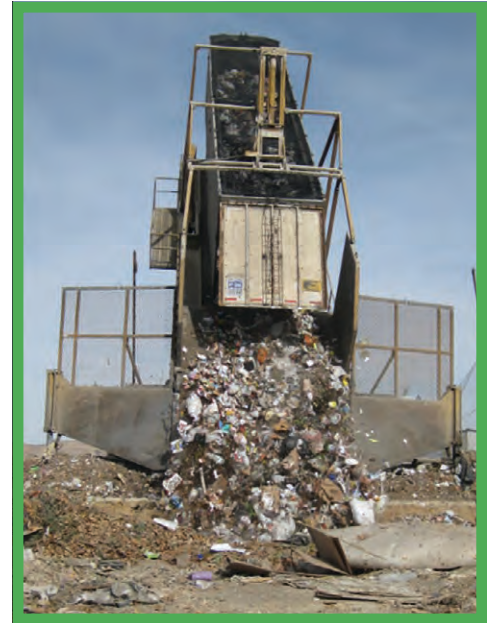
Figure 10: The tipper empties trash into Lockwood Landfill; image from WM
