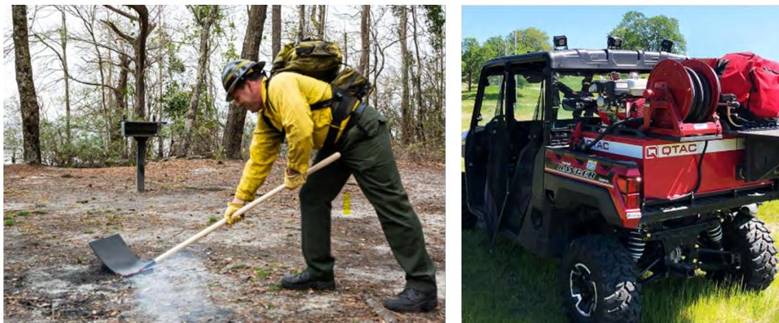
FIGURE 4: FIRE FLAPPER (LEFT) AND UTV WITH SKID SPRAYER (RIGHT)
