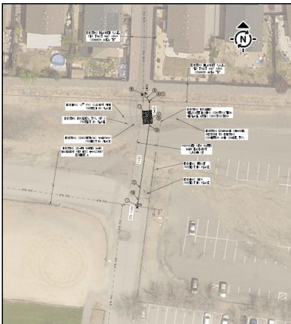
Majority of the work will occur within the existing paved upper parking lot area. All disturbed surfaces will be reconstructed and patched to existing conditions. The existing drainage channel will be restored to its existing condition and grade and the watermain will be protected in place to allow ongoing maintenance of the drainage ditch.
