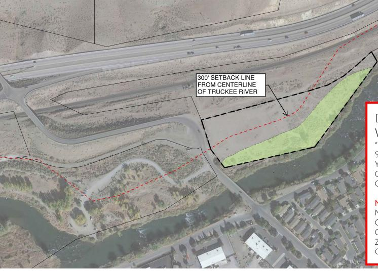
DEVELOPMENT CODE: WCC SECTION 110.222.10(C) "STRUCTURAL SETBACK. NO PERMANENT BUILDING STRUCTURES SHALL BE ERECTED WITHIN THE 100-YEAR FLOODPLAIN, OR WITHIN 300' OF THE CENTER OF THE TRUCKEE RIVER, WHICHEVER IS GREATER.
