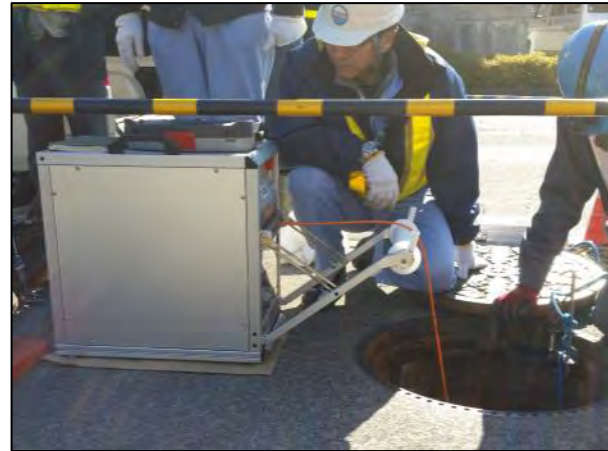
Portable Electro Scan Reel Platform being deployed in remote access sewers in Japan.
