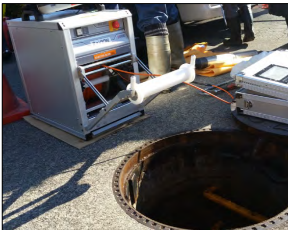
Portable Electro Scan Reel Platform for remote access locations, such as Right-of-ways and easements.
