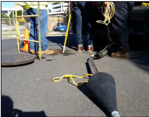
Electro Scan ES-620 probe and Funnel Cone preparing to enter a manhole.
