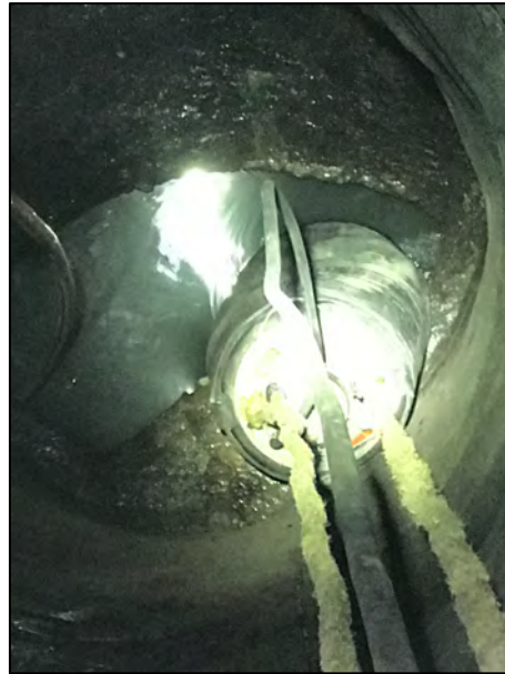
Plug inserted in 24" CIPP lined sewer mains in the City of Houston to surcharge pipe for 360-degree Electro Scanning Testing of pipe wall.
