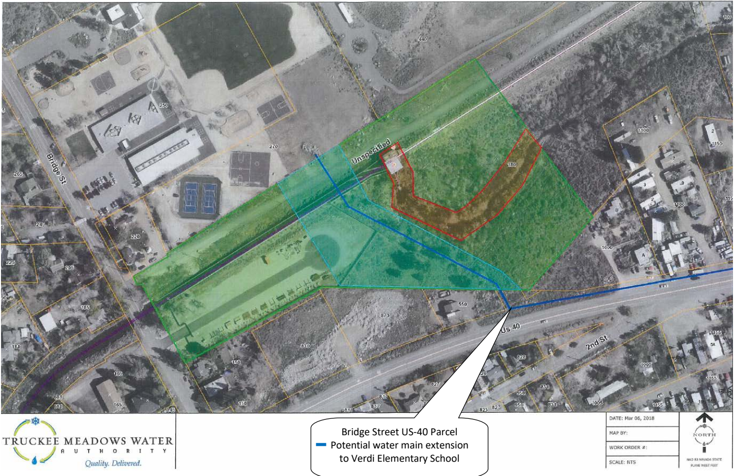
Figure 9: Bridge Street/US-40 Potential Water Main Extension
